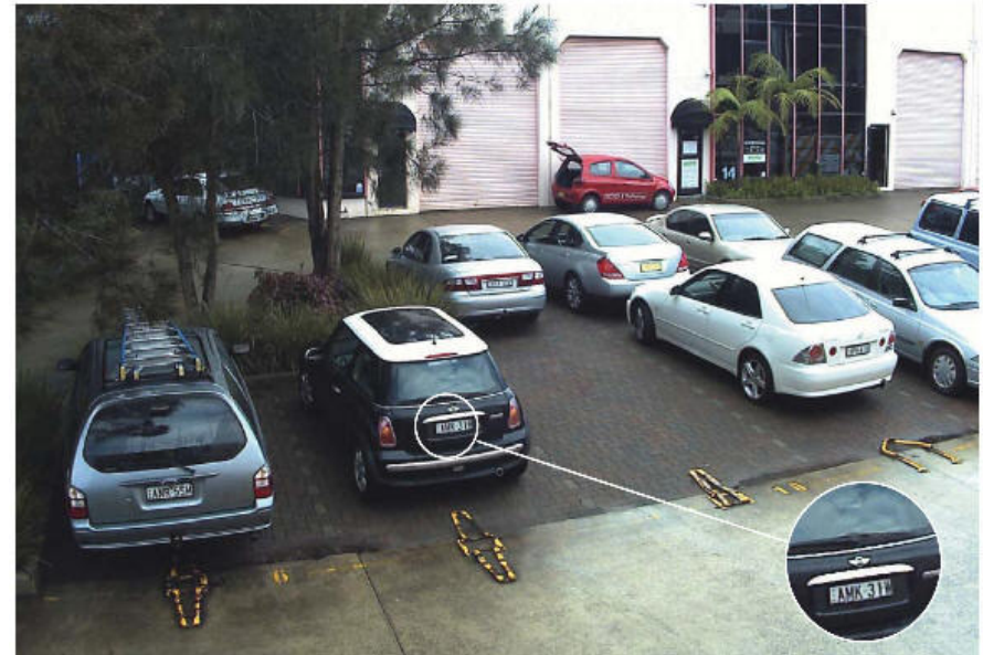
ArecontVision 3megapix camera with Tamron F1.4 lens. Recorded at 2044x1536
