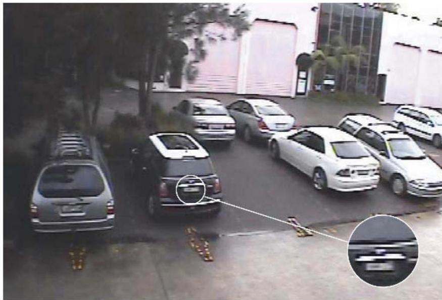
PAL DVR image. Quality camera with Fujion F0.95 lens. Recorded at 704x576
